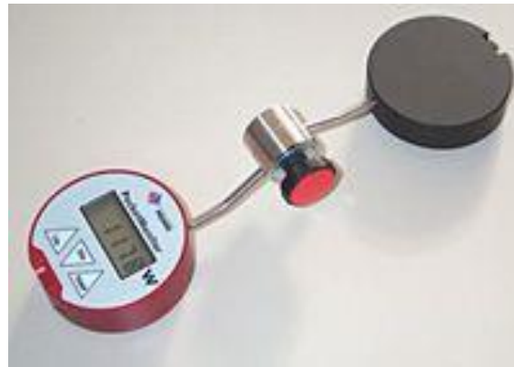
Figure 29 Primes laser power Pocket Monitor PMT 05P
