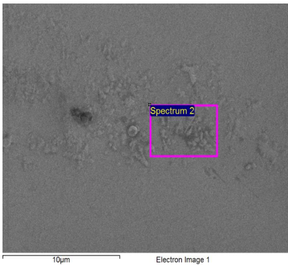
Figure 82 EDS Area 2 Analysis of MMC Sample 3, Sectioned Horizontally
