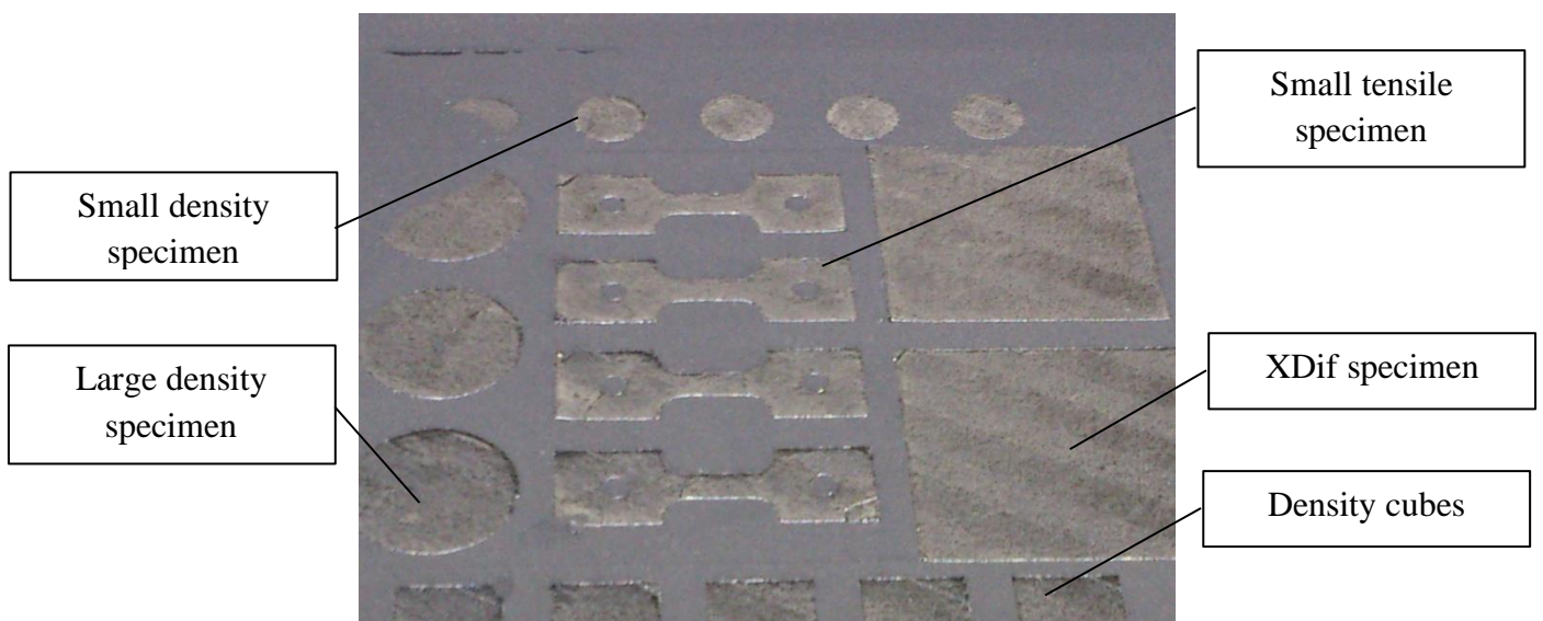
Figure 18 Initial Test Samples. Aborted after approx. 1.5mm
